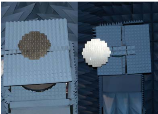
Figure 7 – X-band Waveguide Array Antenna at centered and lateral offset positions
