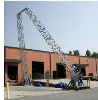
Gantry undergoing factory testing
