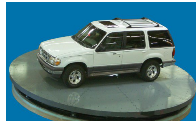
NSI rotator undergoing factory testing
